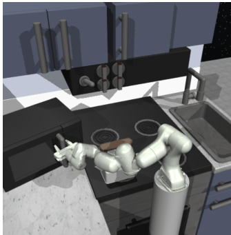
Figure 10: Franka Kitchen environment. In the environment, the robot need to complete 4 subtasks in sequence: open the microwave, move the kettle, flip the light switch, and slide open the cabinet door.
